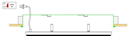
STEP 4: Lift the heater into the FME ensuring the brackets are to the side of the mounts
